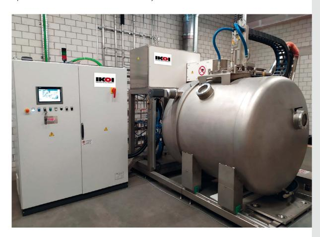
ALS- AcidLess Separation® is a pre-refining equipment to remove silver and volatile elements from Au/Ag/Cu alloys using vacuum distillation technology.
