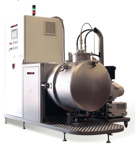
Prime Refining Unit removes silver and volatile elements from Au/Ag/Cu alloys using vacuum distillation technology.
